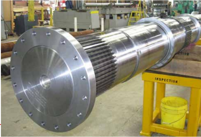
Press Shaft with Induction hardened ppines
