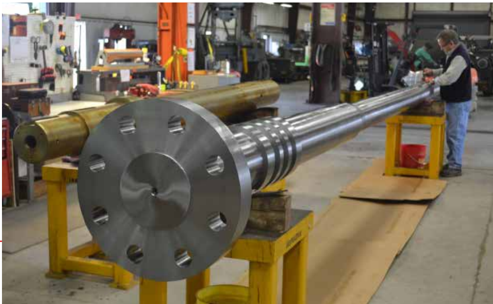
414.75" long Hydroelectric Turbine Shaft for retrofit
