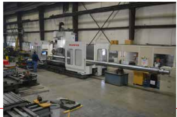
Screw shaft sssembly in the 6-axis mill for keyways - including one 390" long keyway
