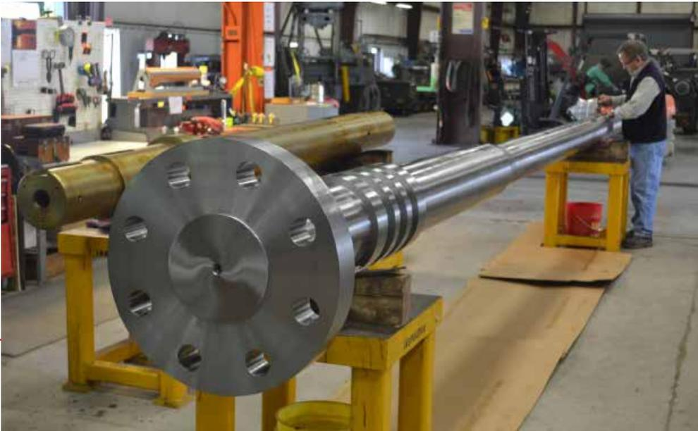
**Hydroelectric Turbine Shaft**
