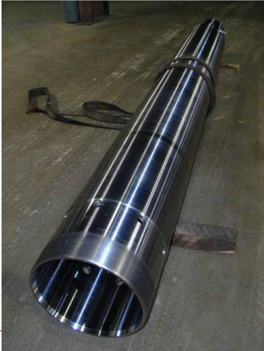
Down hole drilling tube
