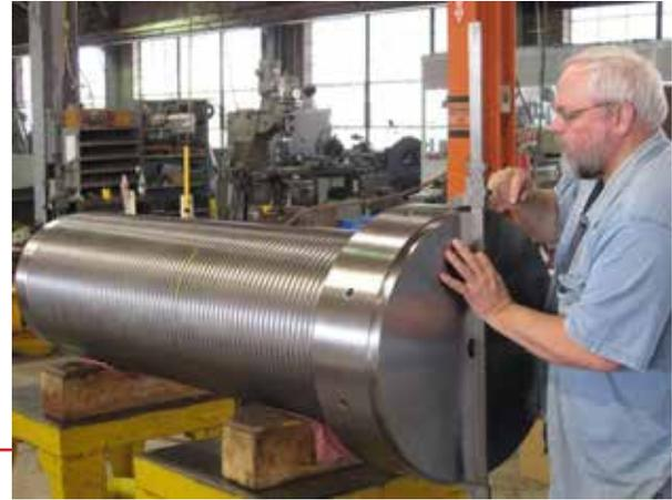
Reversed engineered machine adjustment screw, nitride
