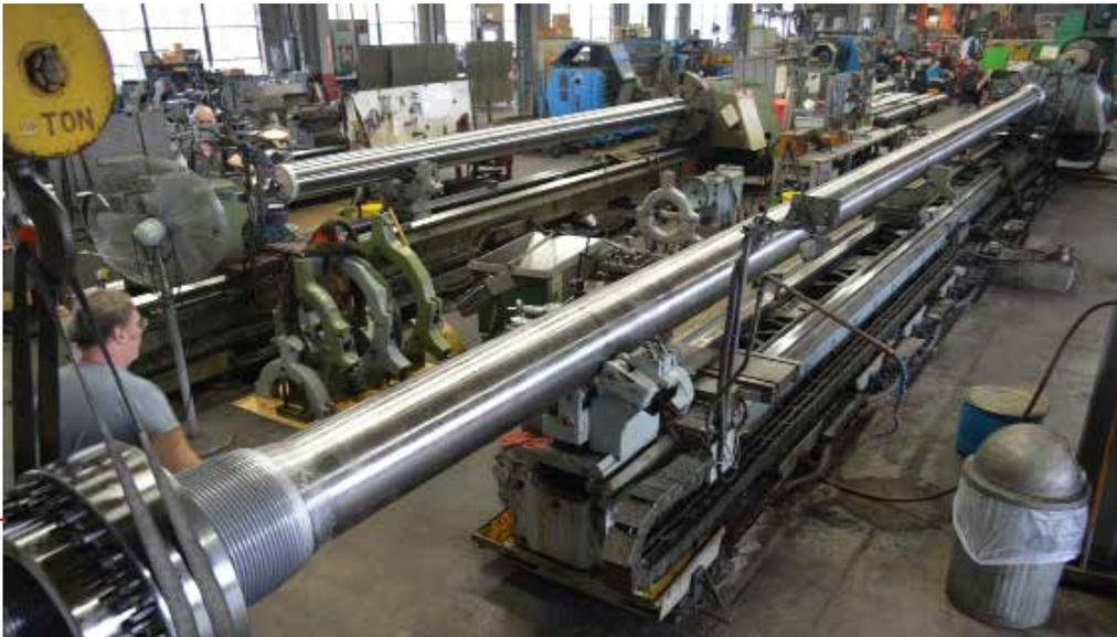
Testing a nut on the bar while in the lathe
