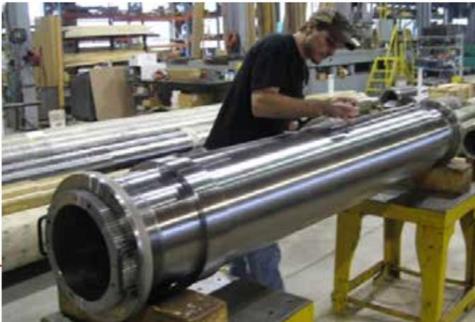
Measuring splines over wires
