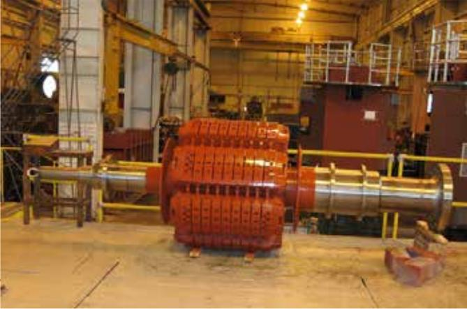
**Electric Rotor Shaft
