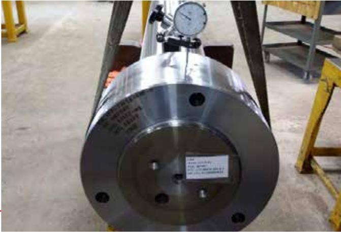
Trying nuts on tie bars to assure fit & measuring the clearance with an indicator
