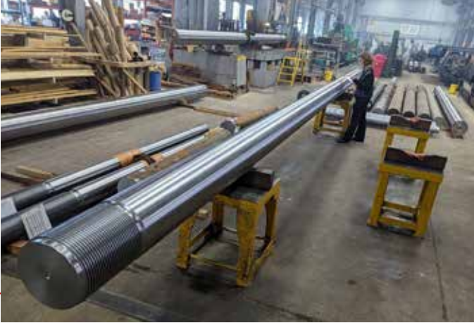
12" diameter x 446" long shaft for friction welding machine
