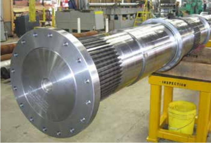
Press Shaft with Induction hardened ppines
