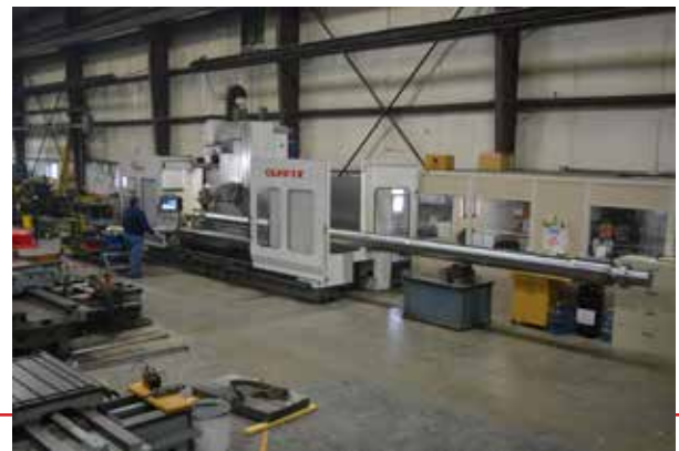
Screw shaft assembly in the 6-axis mill for keyways - including one 390" long keyway
