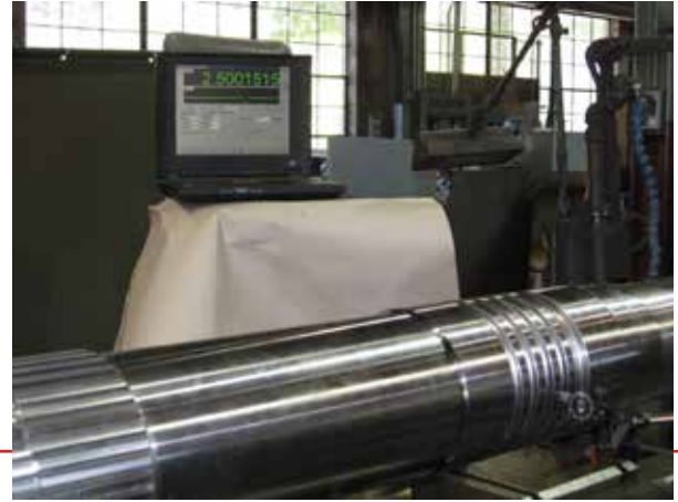
Measuring groove locations with laser
