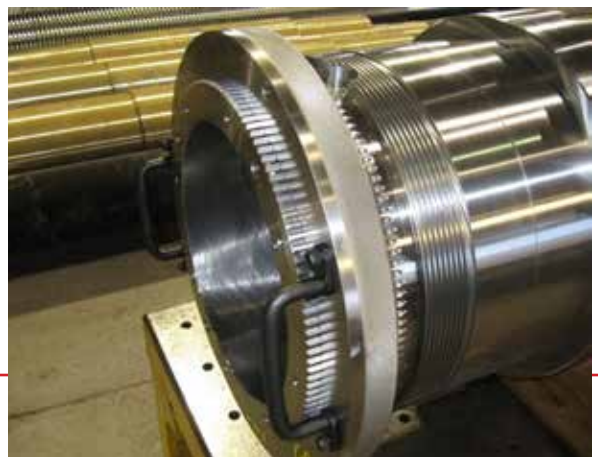
Go spline gage on machined part
