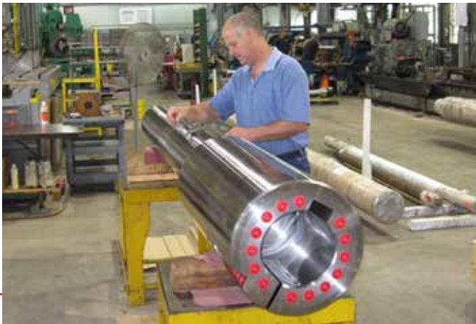
Derive Shaft with internal keyway
