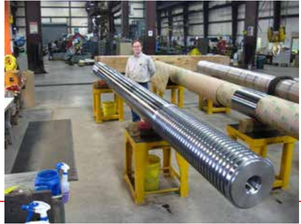
Two-platen die cast tie bar featuring close tolerance groove positions
