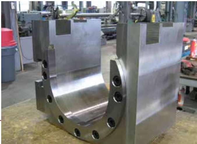
Replacement die carrier for aluminum extrusion press
