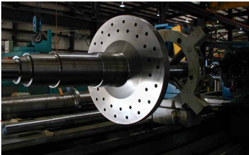
Drilling Flange holes with live tooling CNC lathe
