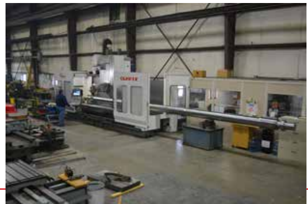
Screw shaft ssembly in the 6-axis mill for keyways - including one 390" long keyway
