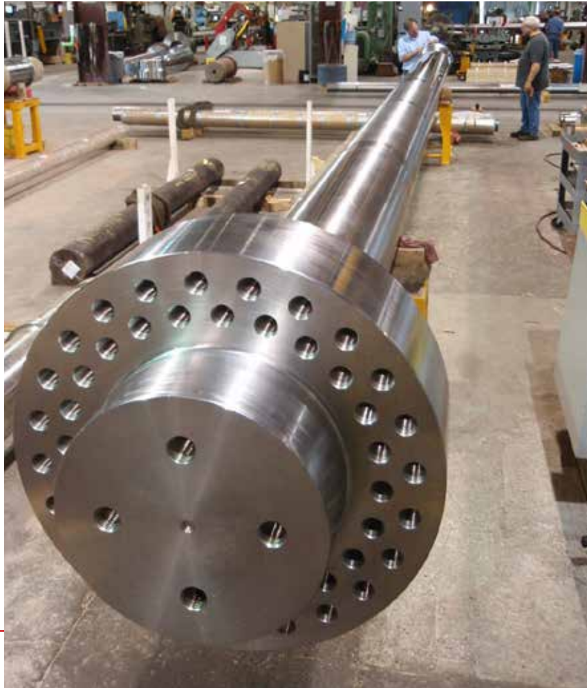
8000T forge press column, 40,000 lbs
