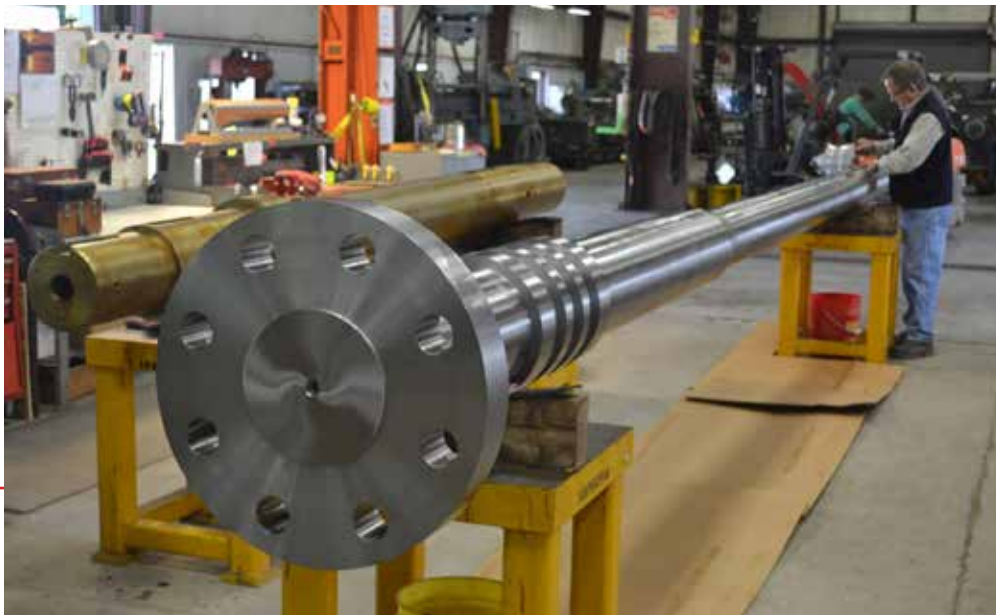
414.75" long Hydroelectric Turbine Shaft for retrofit
