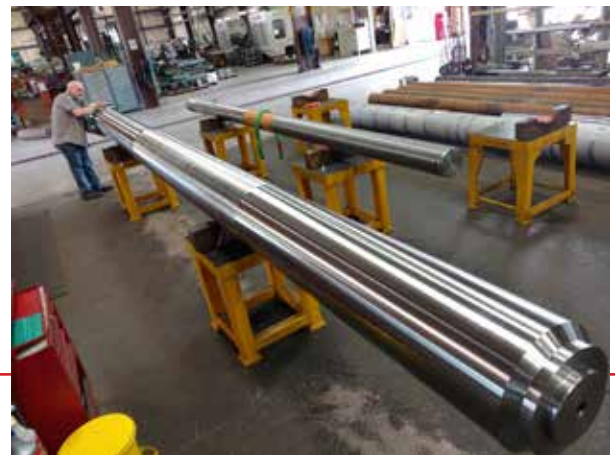
16rms - 0.4Ra um plished surface
